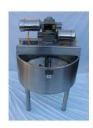
but at a 25-gallon nominal capacity, is perfectly sized for smaller volume producers like laboratory and products development applications. The unique dual agitation configuration, along with heat exchange jacket on the entire cone bottom, provides the operator with the capability to effectively combine and blend ingredients and, in doing so, process the most uniform finished product possible.
